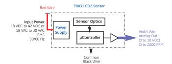
The T8041 is a CO2 transmitter designed to be installed in HVAC return air ducts. This product offers simplicity in design and installation. Available with analog 0-10V output only. Includes mounting hardware and installation instructions
